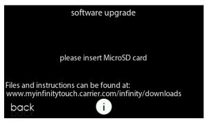
• If the .hex file is stored properly on the MicroSD device, this screen will appear. If the screen says, "Please insert MicroSD Device", remove the MicroSD device and re-insert. If it still does not show the screen, below, go back to the download part and retry.
